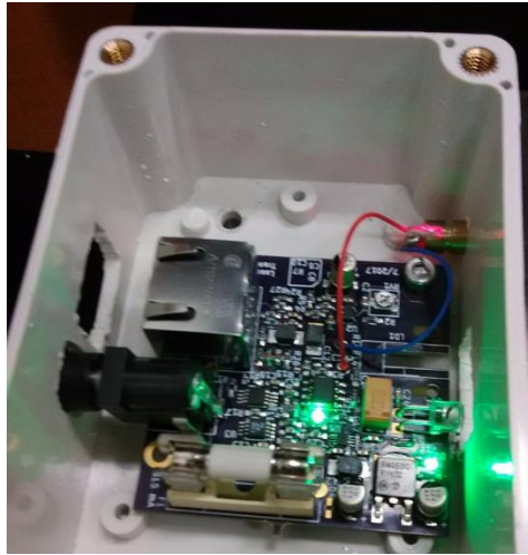
Figure 8.4 The final laser Ethernet transceiver design.
