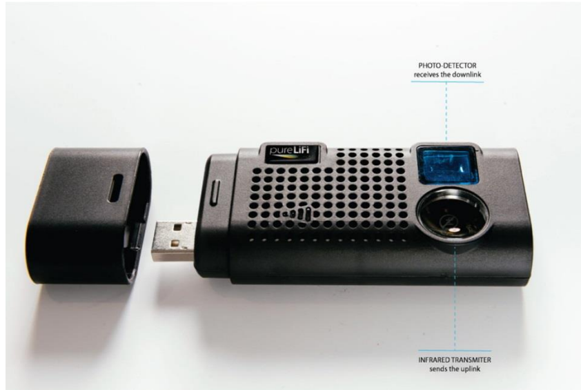
Figure 2.2. The Lifi-X Dongle as produced by PureLifi for their 2017 product release.
